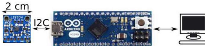
Figure 3.4: Diagram of the data processing of the accelerometer (LIS3DH, Adafruit Industries). The measured data were sent via I2C-bus to a micro controller of type ATmega8 integrated on an Arduino board. The processed data were read out with a computer.
